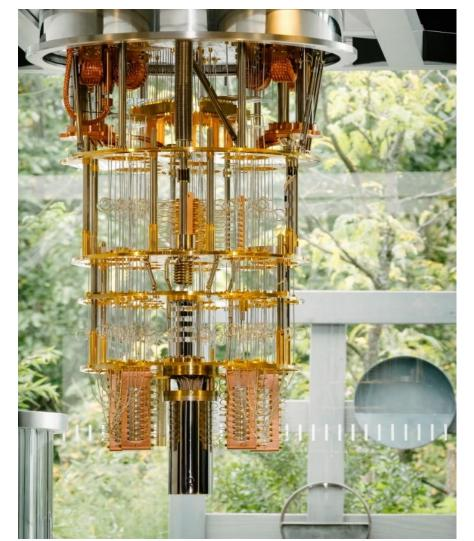
IBM 53-qubit superconductor-based quantum computer
